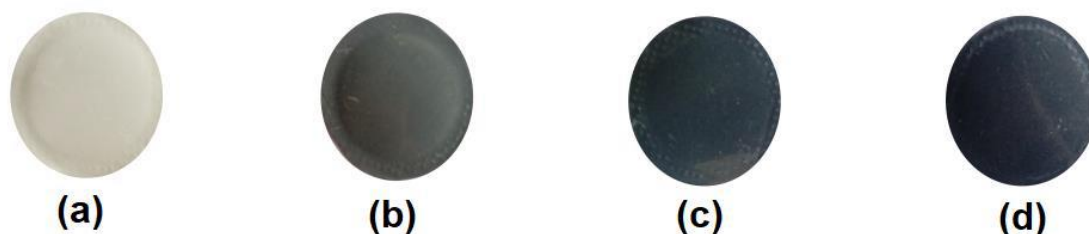
Figure 3 Images of the asymmetric MMMs containing a) 0 wt.%, b) 1 wt.%, c) 3 wt.%, and d) 5 wt.% of MWNT-O.
