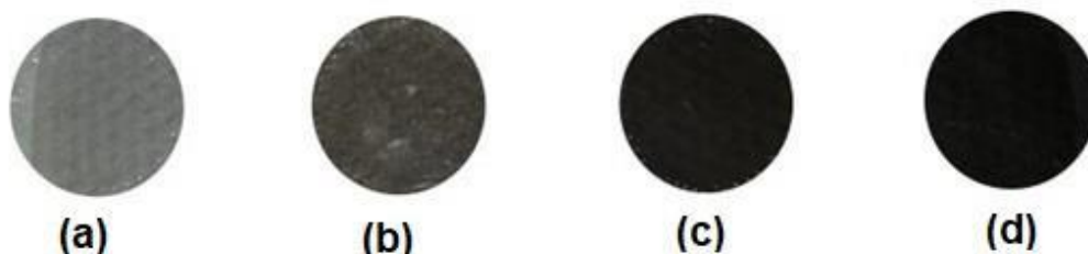
Figure 2 Images of the symmetric MMMs containing a) 0 wt.%, b) 0.1 wt.%, c) 0.5 wt.%, and d) 1 wt.% of MWNT-O.
