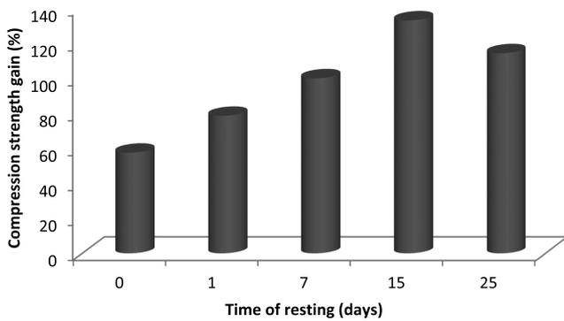
Fig. 2. Gain in the compressive strength of the mini-pellets with the increase of the time of resting of the carbon nanotubes dispersed into the sodium silicate, afterwards added to the iron ore fines for pelletizing. The gain is relative to a reference sample prepared without the addition of carbon nanotubes.
