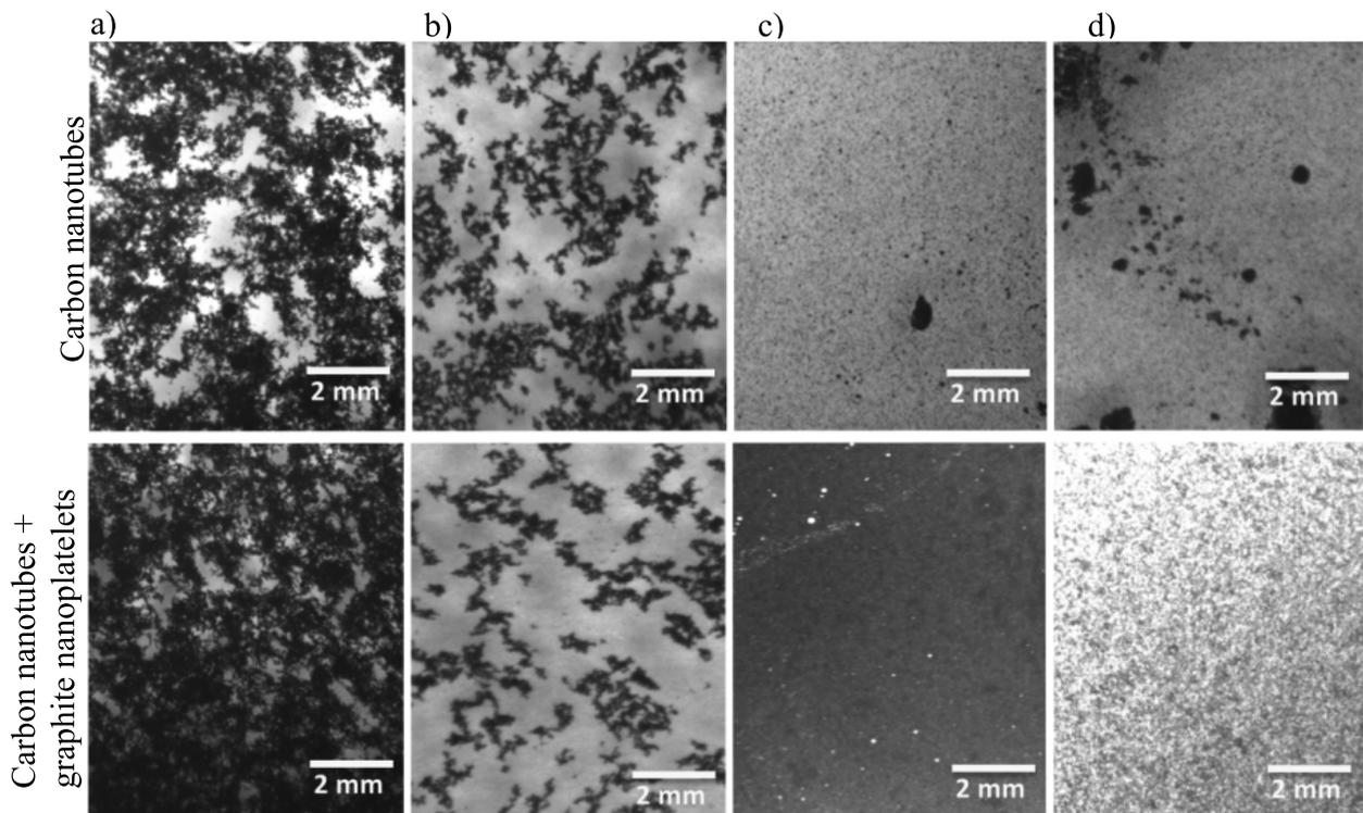
Fig. 4. Stereoscope images of the carbon nanotubes and graphite nanoplatelets into the sodium silicate without dispersion (a) and dispersed after: immediately (b), 15 days (c) and 25 days (d).
