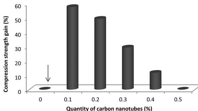
**Fig. 1.** Gain in the compressive strength of the mini-pellets with the increase of the carbon nanotubes quantity on the silicate. The gain is relative to a reference sample of mini-pellets prepared without the addition of carbon nanotubes.
