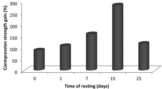
Fig. 3. Gain in the compressive strength of the mini-pellets with the increase of the time of resting of the carbon nanotubes and graphite nanoplatelets dispersed into the sodium silicate, afterwards added to the iron ore fines for pelletizing. The gain is relative to a reference sample prepared without the addition of carbon nanotubes and graphite nanoplatelets.
