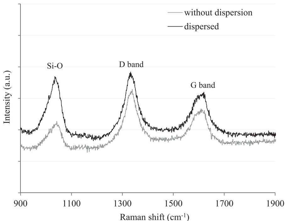
Fig. 5. Raman spectra of the nanomaterials dispersed into sodium silicate before and after the use of the ultrasonic processor.
