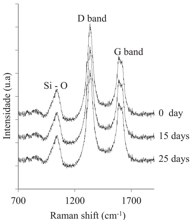
Fig. 6. Raman spectra of the nanomaterials dispersed into the sodium silicate with different time of resting.
