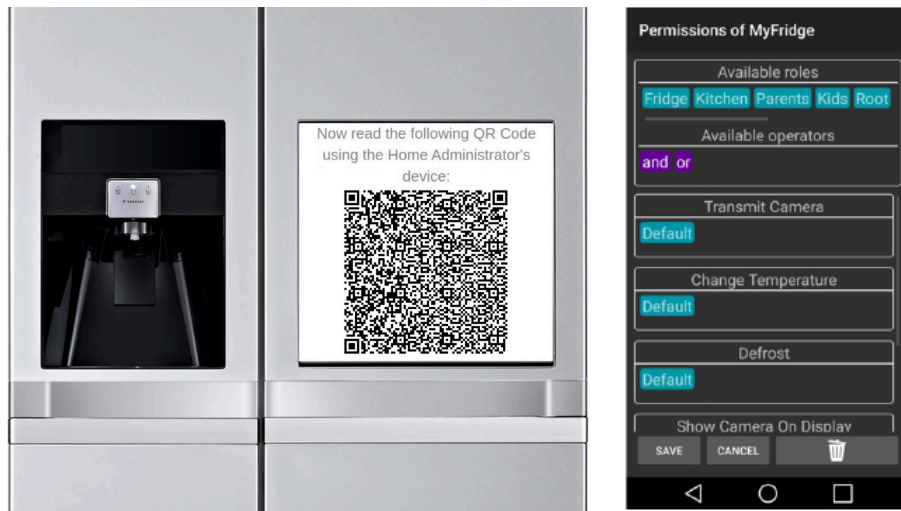
Figure 6.5: The fridge displays a ciphertext to the user (left). Then the user sets the fridge's attributes access control policies (right).
