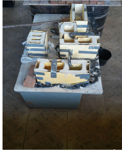
Figure 17: Formworks filled with the mix. Picture taken by Cléber Eustáquio
