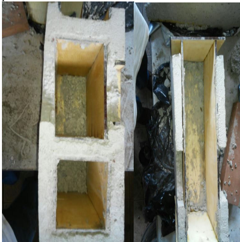
Figure 21: Standard and bond beam blocks - top view. Picture taken by Cléber Eustáquio.
