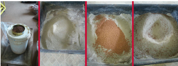
Figure 16: From left to right: Aggregate sifting; preparation of sand and concrete; inclusion of the aggregates and mass mixing. Picture taken by Cléber Eustáquio.
