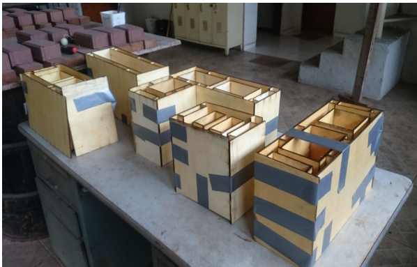
Figure 15: Formworks assembly at the lab. Picture taken by the author.
