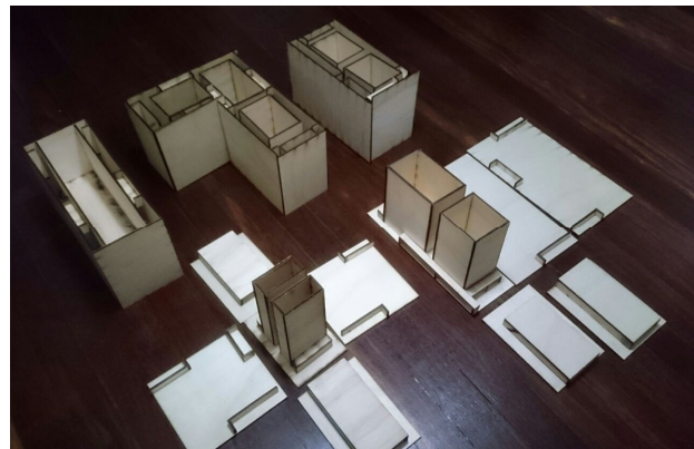
Figure 13: Finished formworks before being coated with varnish. Picture taken by the author.
