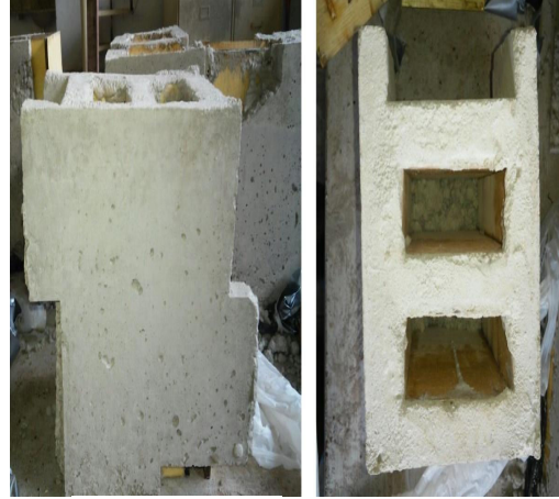
Figure 22: Half block finished. Picture taken by Cléber Eustáquio.
