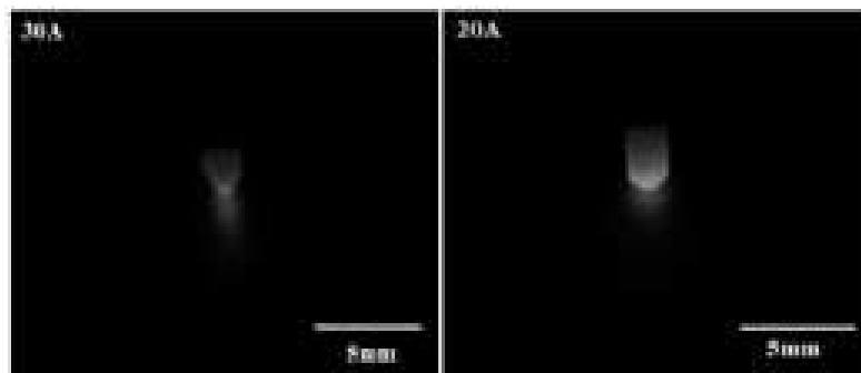
Figure 4. Images of the electric arc for the lower currents.
