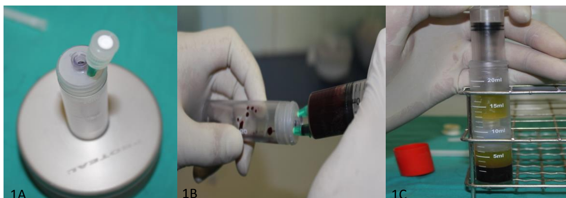
Figure 1. Closed system used in the preparation of platelet rich plasma. 1A: insertion of a 0.22μm filter needle in the embolus port; 1B: transference of blood into the Proteal® tube; 1C: extraction of PRP by coupling a syringe and using the Push.Out® system.
