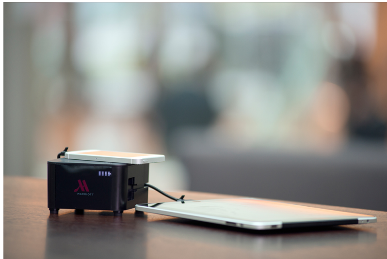
Figure 2.1. Qi Transmitter charging a cellphone (Source: WPC).
