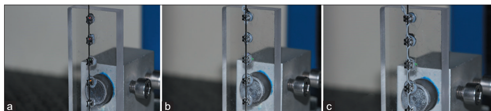
Figure 1: Frictional resistance test carried out for the groups: (a) without elastomeric chain; (b) elastomeric chain under the wire; (c) elastomeric chain over the wire.
