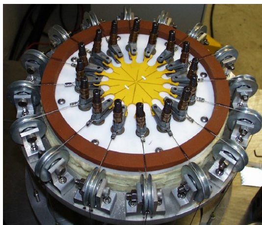
Figure 2-19: Biaxial tensile test apparatus for a circular specimen stretched radially.
