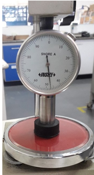
Figure 3-1: Rubber shore hardness test on a type A durometer
