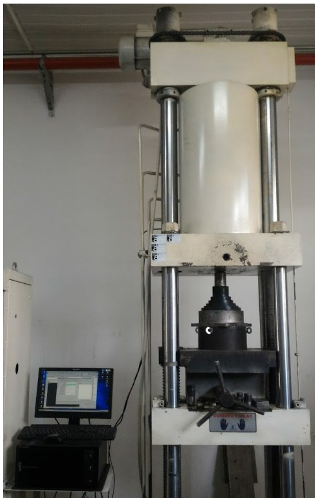
Figure 3-19: Assembly for the axial stiffness test
