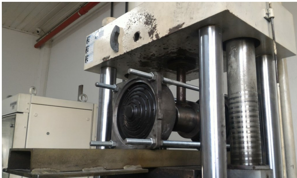
Figure 3-22: Assembly for the radial stiffness test
