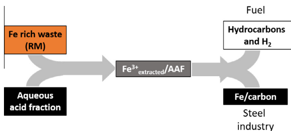
Fig. 1. Schematic representation of the 2W2P (two wastes two products) process.
