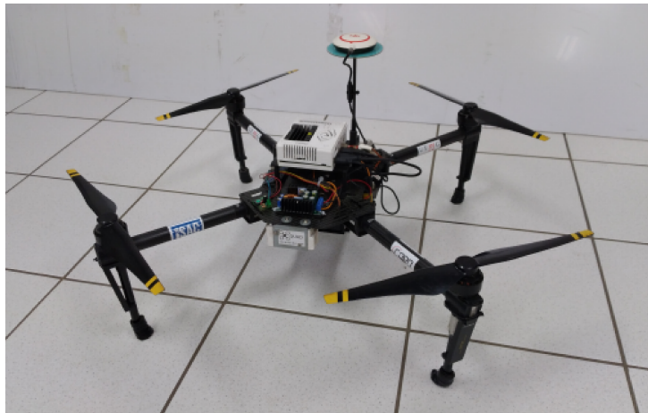
Figure 1.2: Picture of the DJI M100 drone used in the experiments.
