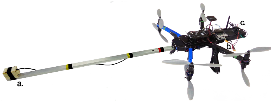
Figure 13. Close up of chosen Unmanned Aerial Vehicle (UAV): X8+ from 3DR. Important components are highlighted on the picture. (a) Sensor head with an 1.1 m aluminium boom; (b) companion computer: Raspberry Pi 2; (c) sensor body.
