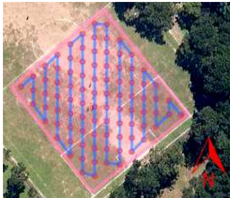
Figure 7. Example of generated path following magnetic north, with 5 m spacing between samples. The pink area is the region of interest, the blue lines are the expected path to be followed and the red circles are the discrete waypoints to visit.
