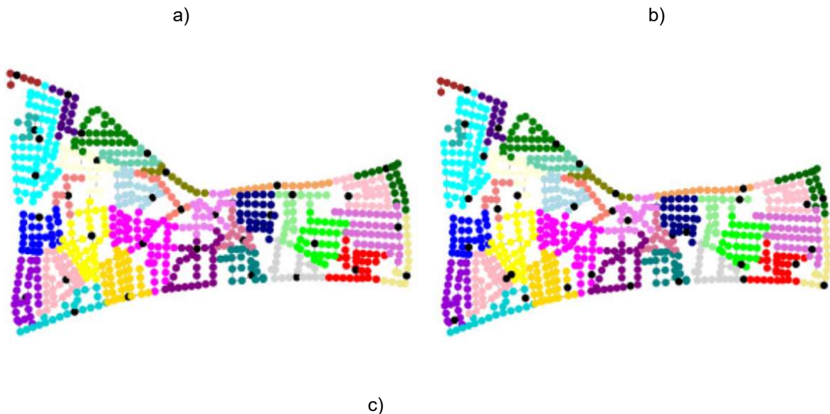
Figure 3.10 - Sensors placed and clusters - L-town network (33 sensors). a) CWSBS. b) BCBS. c) PrBS.
