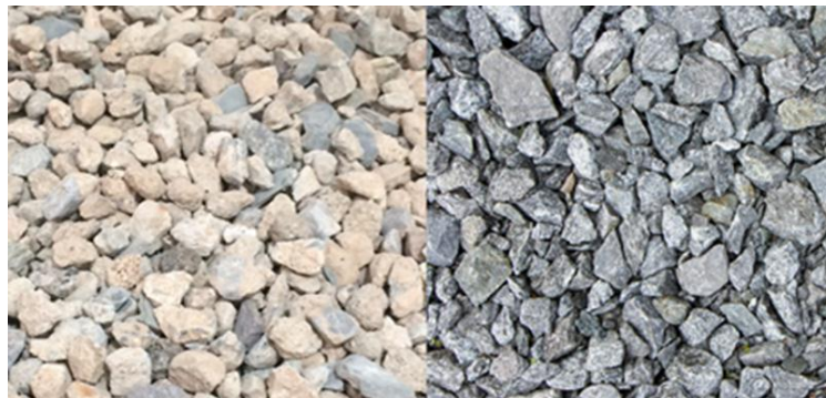
Figure 2: Recycled aggregate concrete (left) and Natural aggregate (right).
