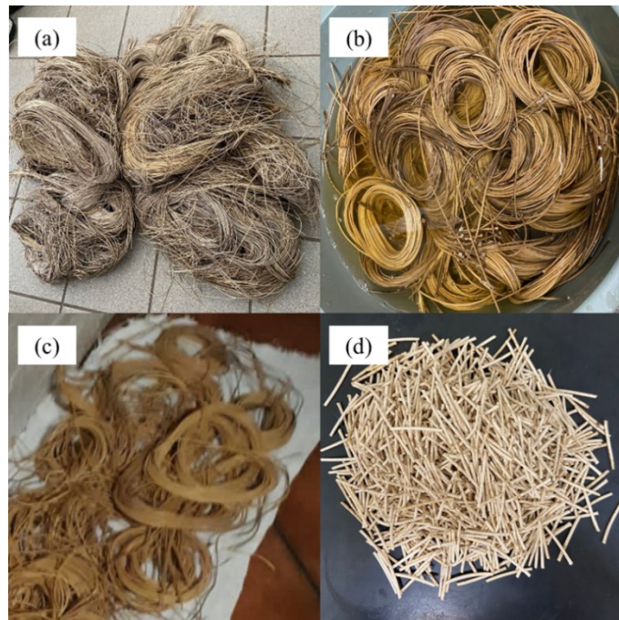
Figure 3.4 - Steps for cleaning and fragmenting PVDF fibers
