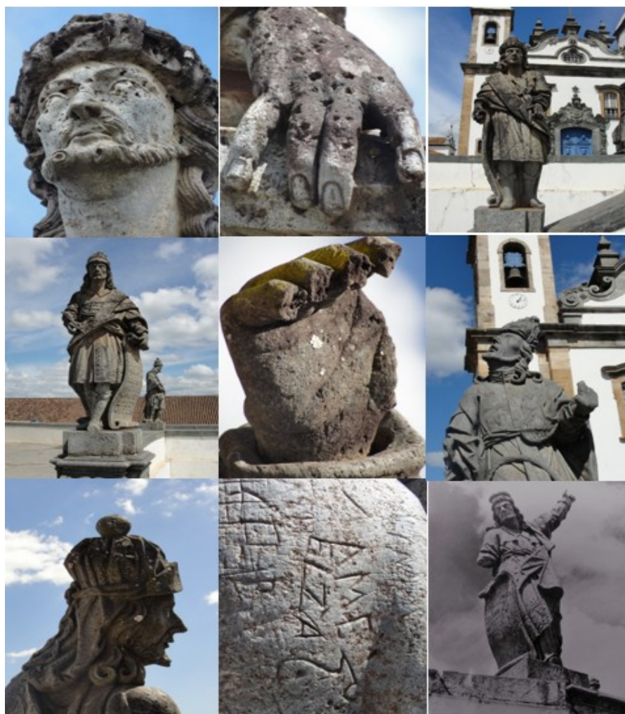
Figure 6: Photographs showing both anthropic and natural vulnerability of the statues symbolizing the prophets present in the Bom Jesus do Matosinhos churchyard. Advanced weathering processes, depredation with breaks in parts of the monument, graffiti, formation of biological accumulations, patina, black crusts, and impurity deposits are noted. The last photo dates from the end of the 19th century, where part of the arm was broken probably due to explosives.
