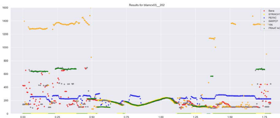
Figure 23 - Raw F_0 estimations of six different PDAs for audio file bfamcv03_202
