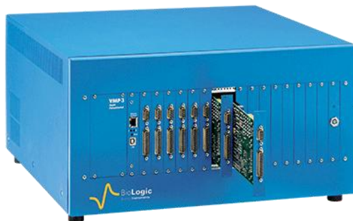
Figura 17. Potenciostato VMP-3 Bio-Logic - Science Instruments.
