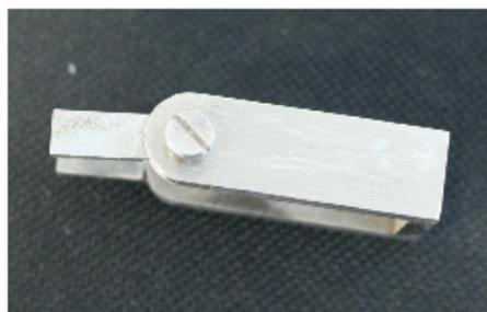
**Fig. 2** The gnathodynamometer with straight bite tip. The bite tip is on the long axis of the load cell
