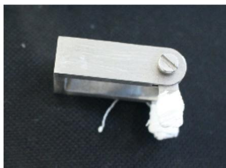
**Fig. 3** The gnathodynamometer with 90° bite tip. The bite tip is on an angle with 90° with the load cell
