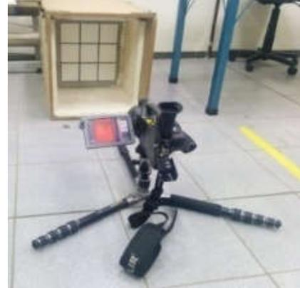
Figure 2. Sample and thermal camera positioned for readings in the thermal box.
