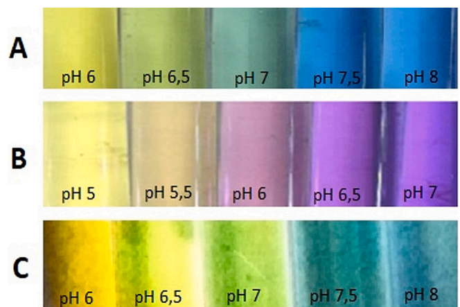
Fig. 1. Standard colors of Bromothymol Blue and Bromocresol Purple at different pH. (A) Buffered standard solutions from pH 6.0 to pH 8.0 containing 0.1% Bromothymol Blue. (B) Buffered standard solutions from pH 5.0 to pH 7.0 containing 0.1% Bromocresol Purple. (C) Buffered standard solutions from pH 6.0 to pH 8.0 containing 0.1% Bromothymol Blue and serum. (For interpretation of the references to color in this figure legend, the reader is referred to the web version of this article.)
