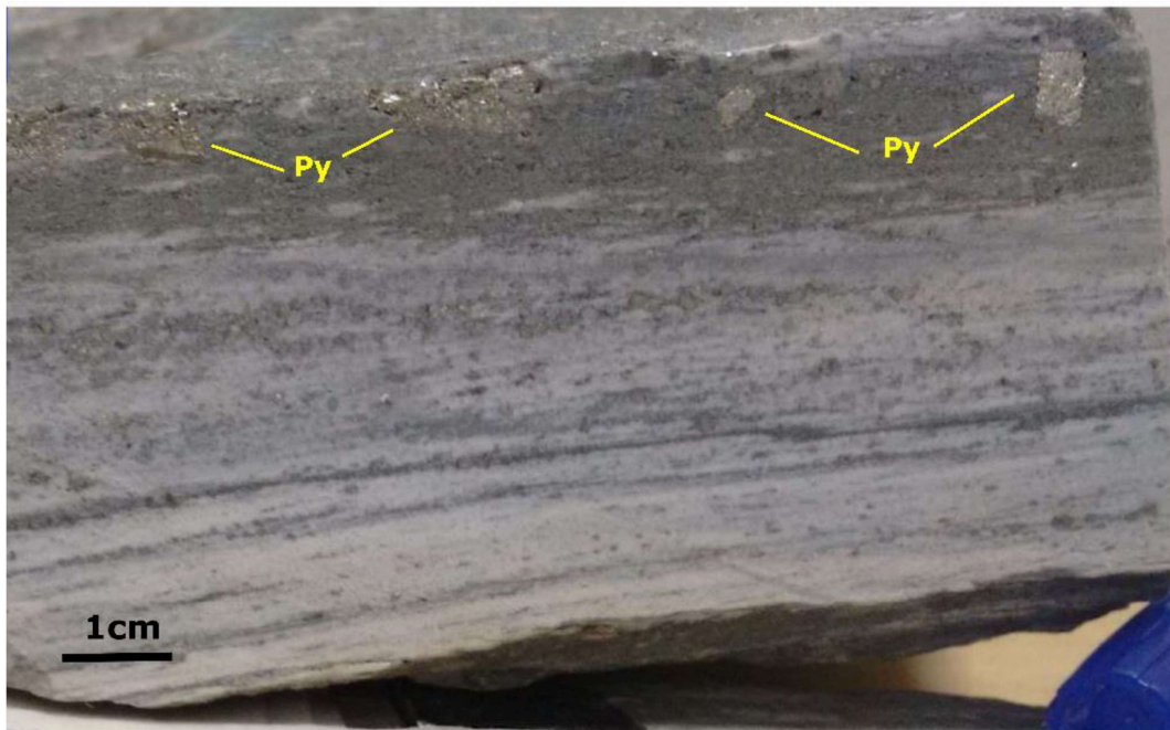
Figura 28: Analyzed sulphidized quartz-plagioclase-veined (silicified) banded schist sample from Pilar deposit. (Py – pyrite crystals and aggregates).
