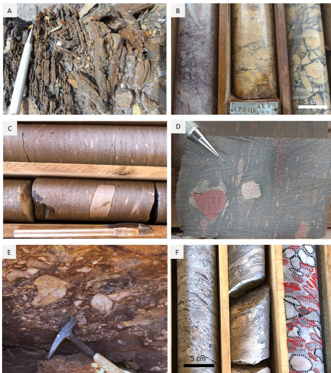
Figure 4.6 A — Folded quartz-itabirite layers from Cauê Formation; B - Drill core sample of brecciated dolostone; C – Intraformational metaconglomerate with cobble of carbonates immersed in matrix ferruginous and carbonate; D – Different shapes and size of carbonate clasts in matrix-supported conglomerate (intraformational metaconglomerate); highlighted dolostone megaclast; E - Matrix-supported metaconglomerate with diversified and deformed clasts associated with the Sabará Group; F - Drill core sample of metaconglomerates imbricated clasts of quartzite (black lines) and BIF (red lines) from Itacolomi Group.
