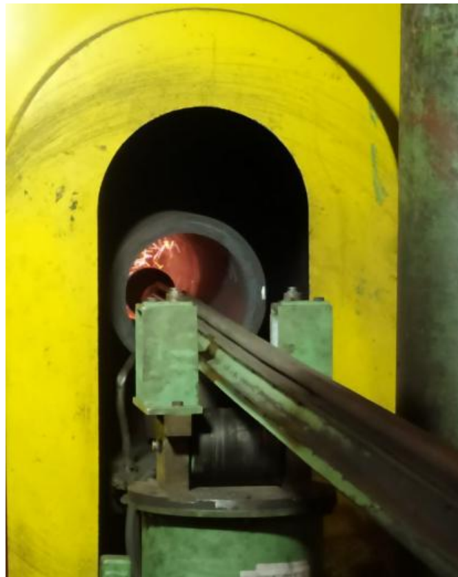
Figure 4.4 - Grinding operation at the inner surface of the pipe.
