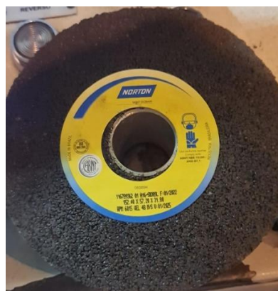
Figure 4.3 - Grinding wheel used in the automatic repair operation on the inside pipe surface.
