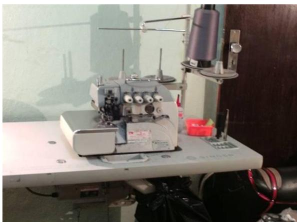
FIGURA 6: Máquina overloque
