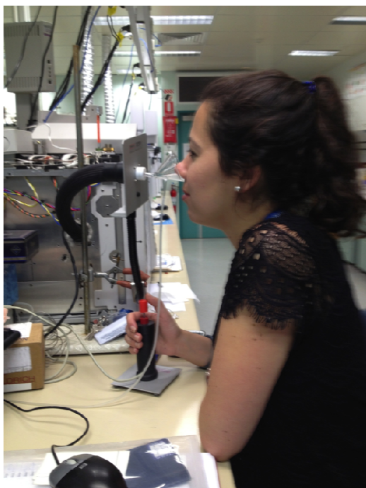
FIGURE 4.1 Picture of a panellist sniffing on the system of GC/FID/O From: own Author, 2014
