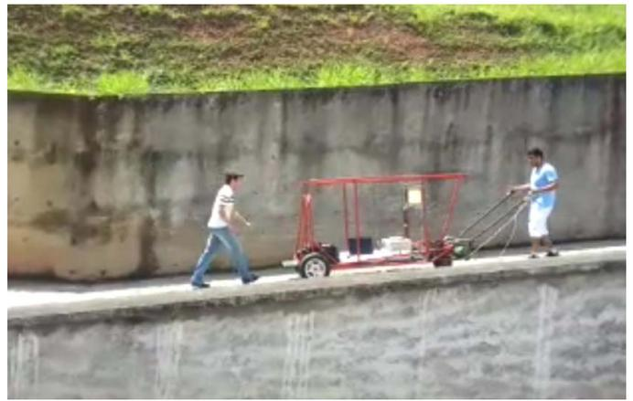
Fig. 12. Vehicle displacement over a 7.8 degrees inclined surface with 120kg
