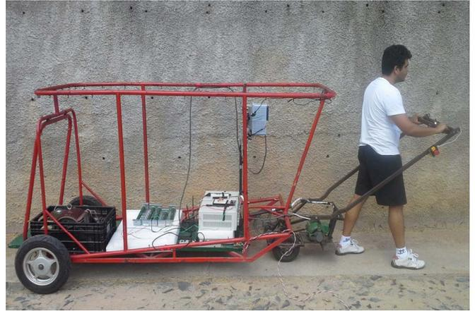
Fig. 1. Side view of the structure and mechanical traction system for electrical load cart, emphasizing the motor, transmission and guidance bar.
