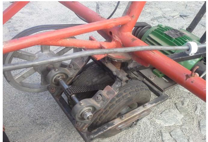
Fig. 2. Double stage transmission system.
