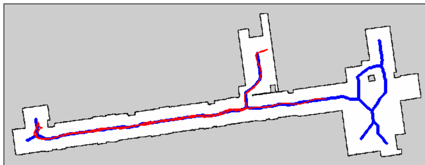
Figure 4.14: Blue thicker line is the GVD and red line is the robot trajectory.
