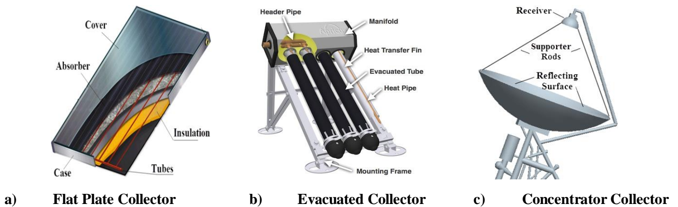
FIGURE 1.2 – The schematic of various types of solar collectors
