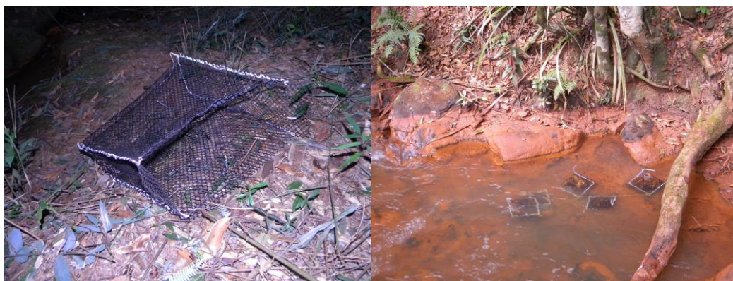
Figure 13 – Collector for lateral litter input (left) and decomposition litterbags incubated in Brucutu stream (right).
