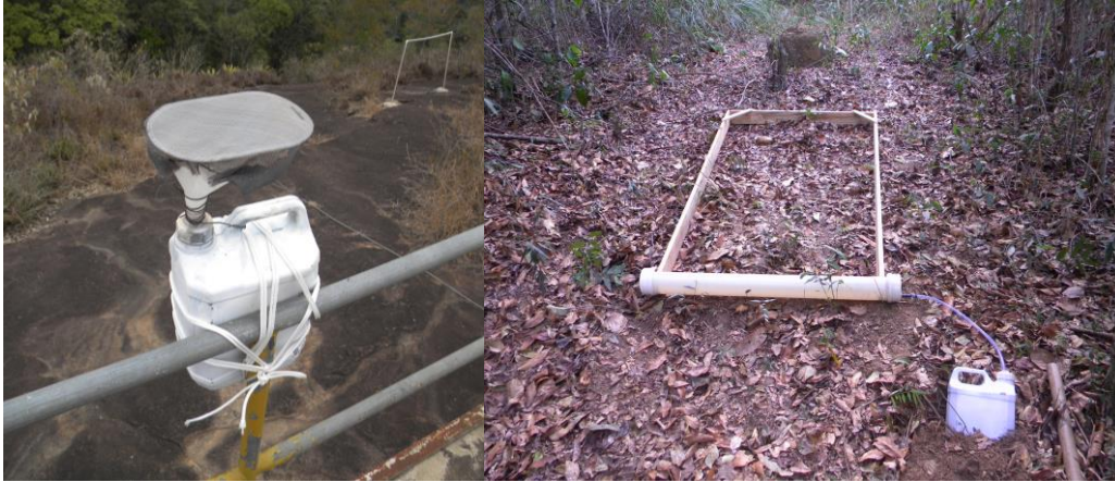
Figure 3 – Collector for wet deposition (left) and runoff (right).
