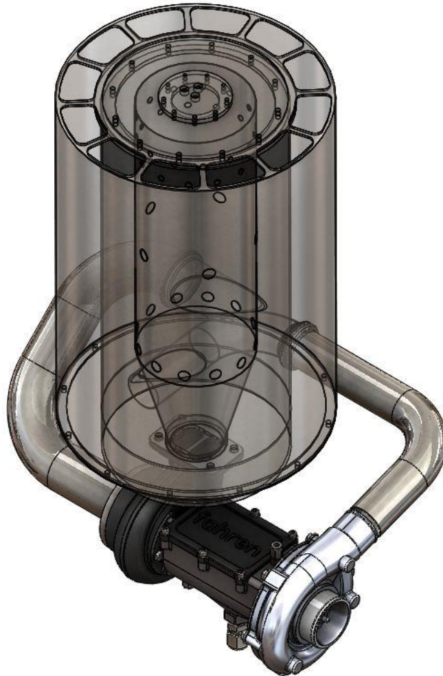
Figure 3 – Initial CAD model for microturbine assembly.
