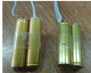
(b) The cells connected in groups of two cells with 3V potential.
