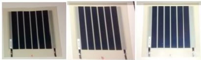
Figure 30 - OPV modules prior to the aging tests
