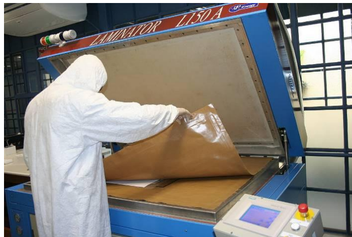
Figure 17 - Laminator used for samples preparation
