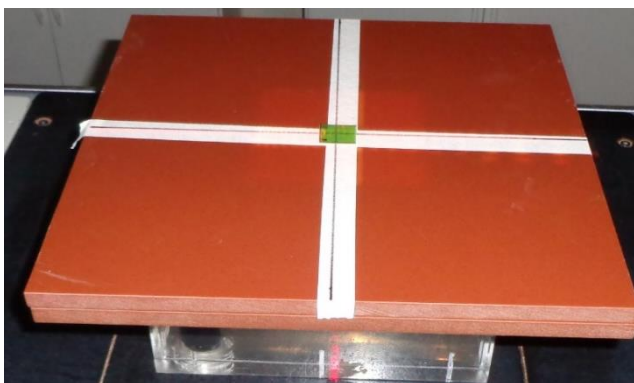
Figura 2-2: Experimental setup of the calibration in solid water
