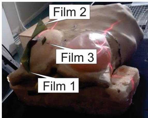
Figura 4-1: Films positioning on thoracic phantom
