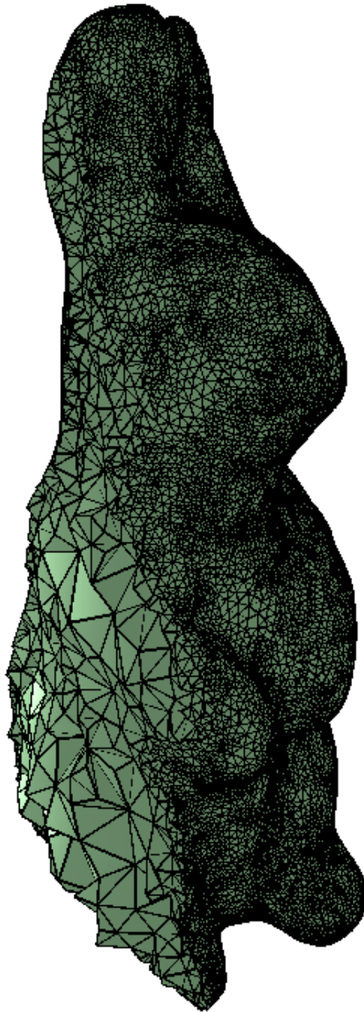
Figure 5.22: A cut in the volumetric mesh of the remeshed rabbit model (Figure 5.19(b))
