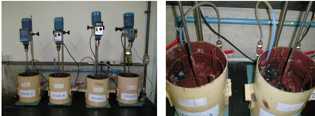
Figure 3.2 – Stirred Tanks used to Carry Out the Second Phase of the Laboratory Tests
