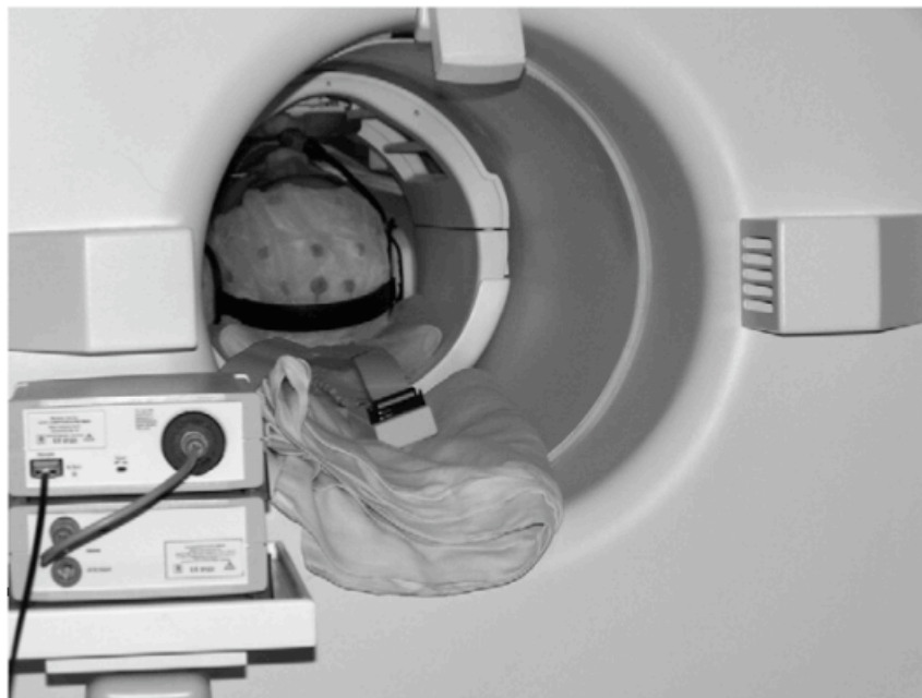
Figure 2.9: The amplifier system placed close to the subject's head inside the scanner (Herrmann and Debener, 2008). The signal is transmitted via optical fiber to a recording room to avoid electromagnetic interference.
