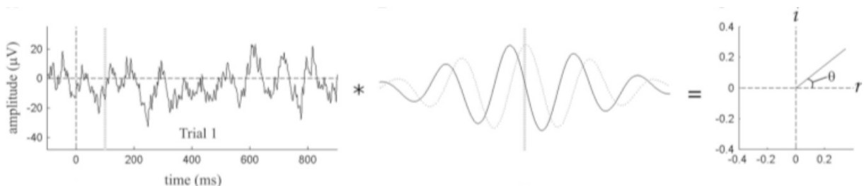
Figure 3.8: Example of an EEG time series convolved with a Morlet function, containing real and imaginary components.
