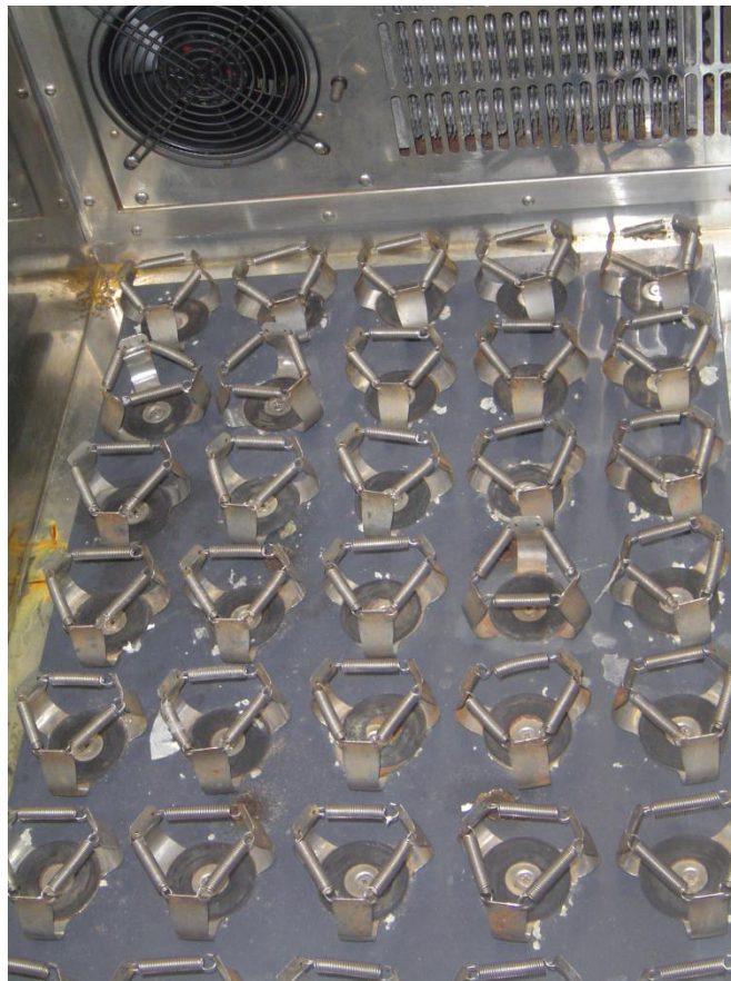
Figura 4.5: Shaker New Brunswick: (a) vista externa, (b) vista interna (DEMET/UFMG).
