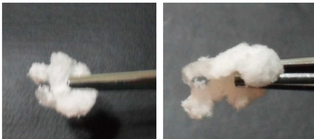
Figure 6.11: Digital images of foam obtained from composite PU/PVA with 25% of BGNP.
