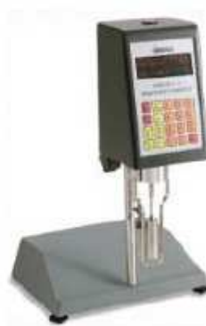
Figura 4.6 – Viscosímetro Brookfield, modelo DV-III. ( www.brookfieldengineering.com ).
