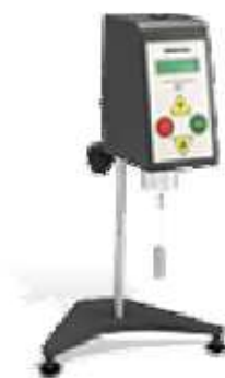
Figura 4.8 – Reômetro Digital Brookfield, modelo YR-1. ( www.brookfieldengineering.com )
