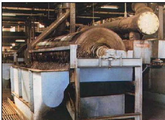
FIGURA 3.9. WRDE – Wet rare earth drum (Arquivo particular do autor, 2006).
