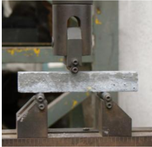
Figure 4.1 – Experimental setup for three-point bending test
