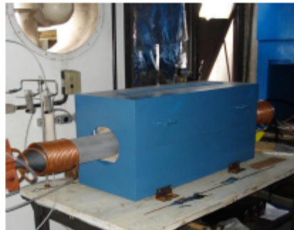
Figure 1. The CVD reactor used for in situ CNT/CNF synthesis on cementitious materials.
