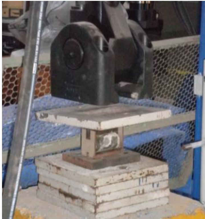
Figure 4.2 – Experimental setup for splitting tensile strength tests
