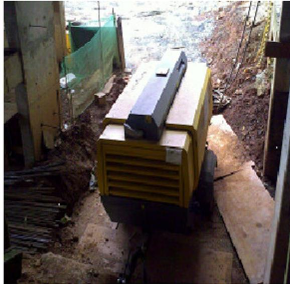
**Foto 11:** Detalhe do compressor central a diesel. (10 bar – 360 pcm).
