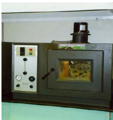
Figura III.4 – Aparelho de RTFOT – Rolling Thin Film Oven Test
