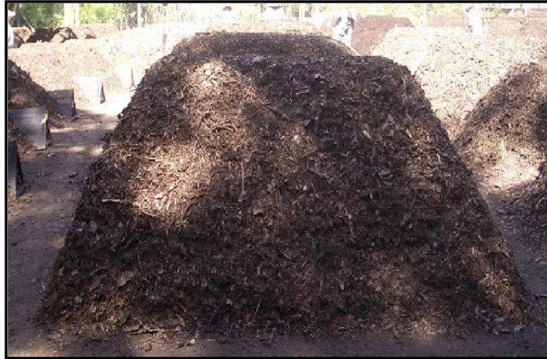
FIGURA 8: PROCESSO DE COMPOSTAGEM DO TIPO WINDROW.
