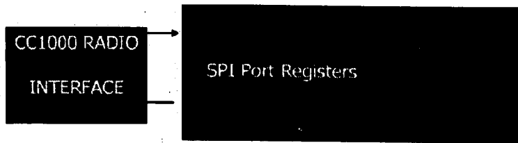
Figure 5.7: Radio driver using SPI.
