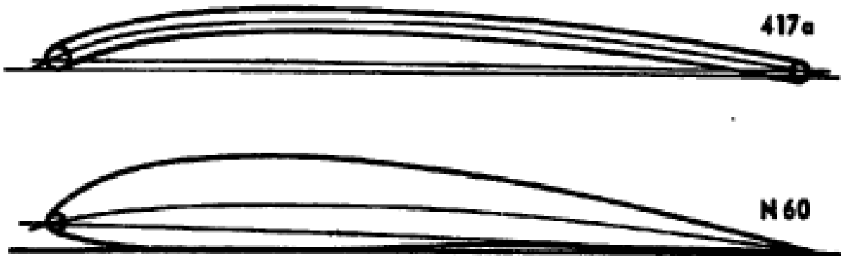
Figure 3.6: Cambered plate '417a' and airfoil N-60, from Schmitz (1942)
