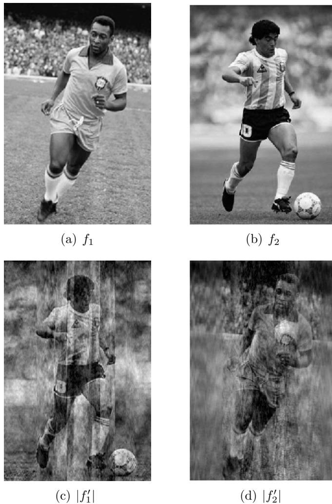
Figure 1.3: Illustration of the process given in equation (1.18); (a) and (b) show the original functions f_1 and f_2 , while (c) and (d) show the absolute values of the resulting functions, f_1' and f_2' , after exchanging their phase in the Fourier domain. Besides adding some noise, the net result is to interchange the pictures, which illustrates how important the phase information is.
