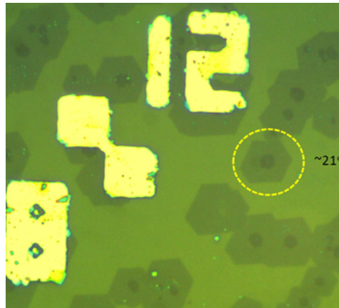
Figure 32 – Optical image of some TBG samples, the circle shows one sample that the angle was measured with the optical image.
