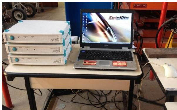
Figura 5.8 – Spider8 600 Hz e laptop com mouse.
